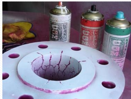
Dye Penetrant Test for detection of surface cracks
