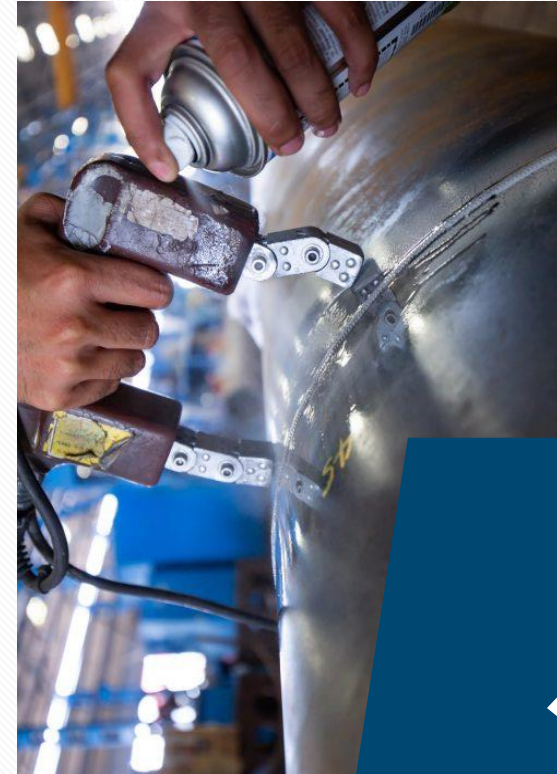
Magnetic Particle Inspection for detection of surface and subsurface cracks
